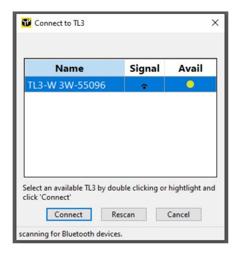
If the TL3 does not appear please make certain that TL3 Bluetooth has been enabled and Windows Bluetooth is working. Note: It is not necessary to pair the TL3 to Windows before using the software.
