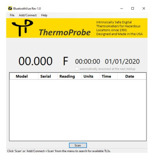
From the BluetoothVue main window select the 'SCAN' button to open the Connection window. The active TL3 should appear in the connection window.
